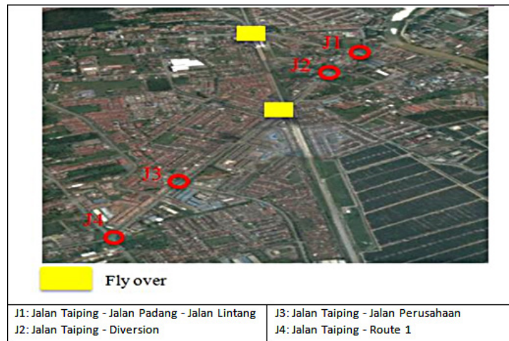
Fig. 3: The changed layout of signalised intersection along Jalan Taiping from six junctions to four junctions following the completion of flyovers.
