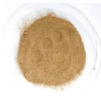
Fig. 2(b): Pulverized MCB
