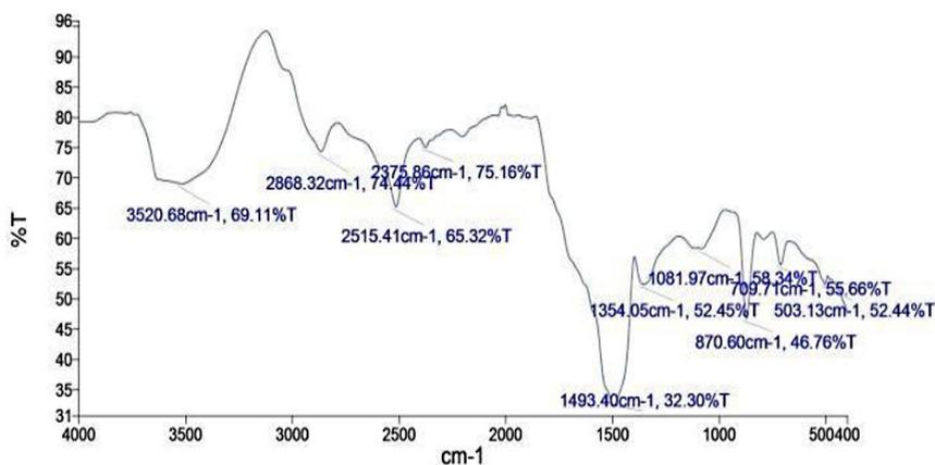
**Fig. 6: Spectrum result of Calcium Hydroxide**
