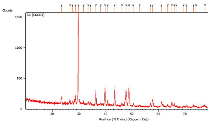
**Fig. 3: Peak profile view of Calcium Carbonate**
