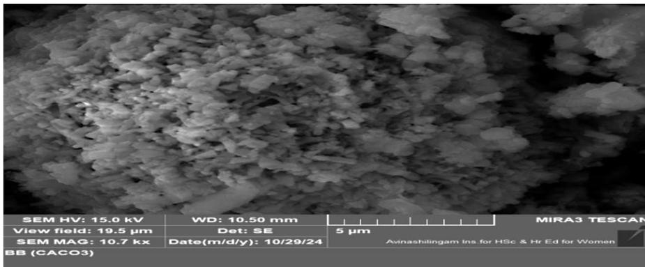
Fig. 8: SEM image of Calcium Carbonate with pores
