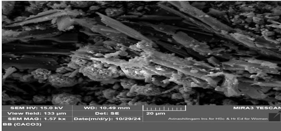
Fig. 7: SEM image of Calcium Carbonate
