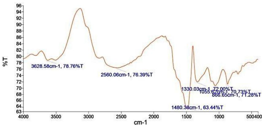
**Fig. 5: Spectrum result of Potassium Hydroxide**
