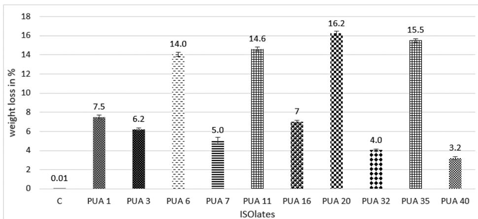
**Fig. 5: Percentage of LDPE sheet weight loss after 30 days of incubation**
